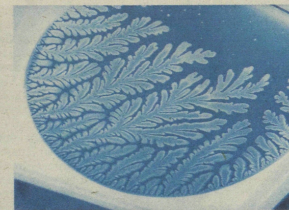
BLUE-DYED glycerine in the U-M experiment shows parabolic tips with side-branching. This array of dendrites is similar to shapes seen in unsuccessful castings of metals.
