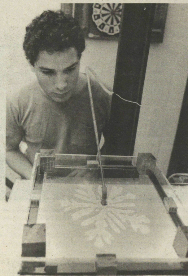
COMPARE THIS PATTERN produced in a physics experiment conducted by senior Tom Mueller with the one on the front cover. The form above — made by pumping air into glycerine squeezed between two plastic plates — is an example of tip-splitting, the most elementary pattern formed at the interface of two systems thrown out of equilibrium. The tip evolves by broadening, flattening, forming a groove and eventually splitting into two new tips that continue to evolve in this fashion. The front cover shows an example of dendritic (tree-like) growth, which is characterized by stable tips that push out and branch. The snowflake-like symmetry is imposed by scoring the lower plate holding the glycerine. The scored lines are analogous to frame, or lattice, of the 2-hydrogen, 1-oxygen water molecule. This lattice imposes the six-sided pattern on the water crystal we call snow. U-M physicist Eshel Ben-Jacob theorized that the tip-splitting and snowflake forms were linked; Mueller and Rob Godbey ('86) joined Ben-Jacob in devising an experiment that supports the theory.
