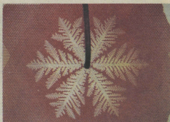
'SNOWFLAKE' in red glycerine. This pattern is created by grooving the lower plate, imposing a condition called anisotropy (see discussion of theoretical model in article) as the water molecule does to a snow crystal. Ben-Jacob and his colleagues predicted mathematically that this shape would occur under given conditions.
