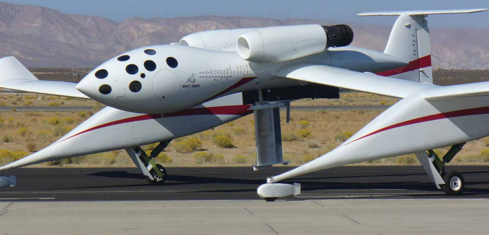
THE WHITE KNIGHT AIRCRAFT WAS USED FOR FLIGHT TESTS OF THE FLEXSYS ADAPTIVE WING (MOUNTED ON UNDERSIDE OF AIRCRAFT AND IN DRAWING BELOW).
