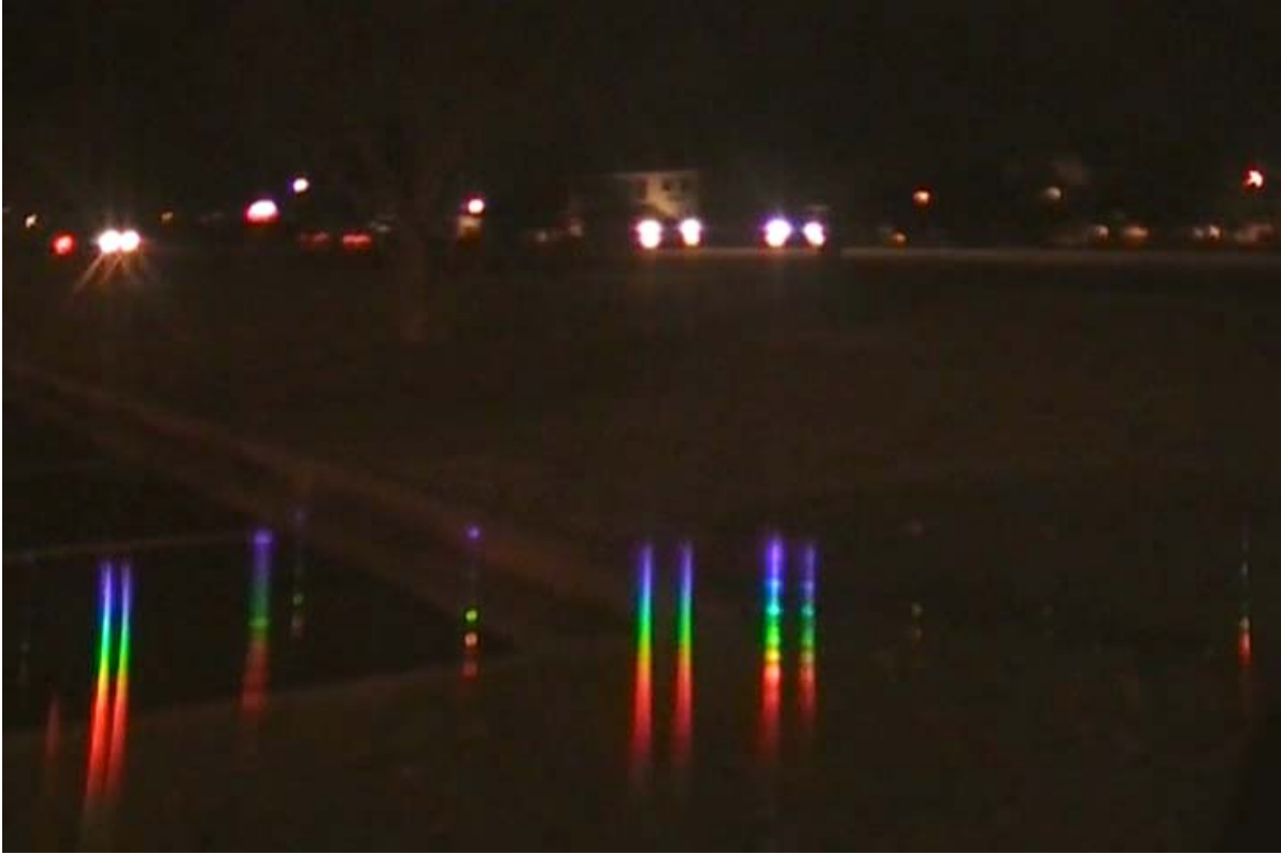
Figure 2. An example video frame, illustrating the appearance of normal and spectrally dispersed headlamp images of TH and HID headlamps. Three pairs of headlamps and their spectra are visible: a TH pair near the left edge, a TH pair near the middle, and an HID pair just to the right of middle. See text for details.
