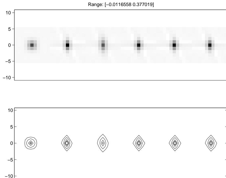
Figure 5.13: Impulse Responses at (-100,-100). From left to right, target, conventional regularization, certainty based regularization, AIMA regularization with \alpha = 0.1 , AIMA regularization with \alpha = 0 , FIIN regularization with \alpha = 0 .
