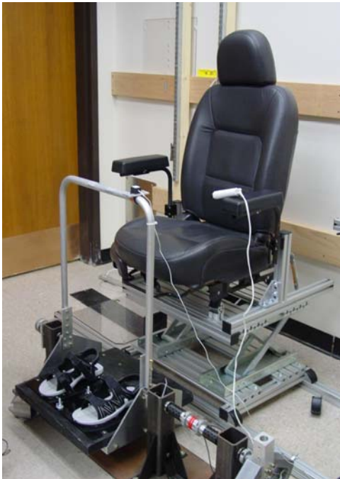
Figure 2.1 Device 1: Ankle-strength-matched platform. This reconfigurable device limits the subject's motion to plantar flexion and dorsiflexion of the ankle. It is capable of presenting programmable loads to the ankle on the same scale as those felt during everyday tasks, such as standing. In the figure, the device is ready for a seated subject but can be reconfigured for standing as well.
