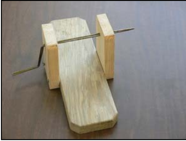
Figure 6.4. A bandage-rolling machine, made of scrap wood and clothes hanger wire, for making rolled sheet bandages
