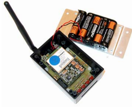
Figure 2-1: A low-cost wireless sensor whose hardware design is optimized for structural monitoring of civil infrastructure systems.
