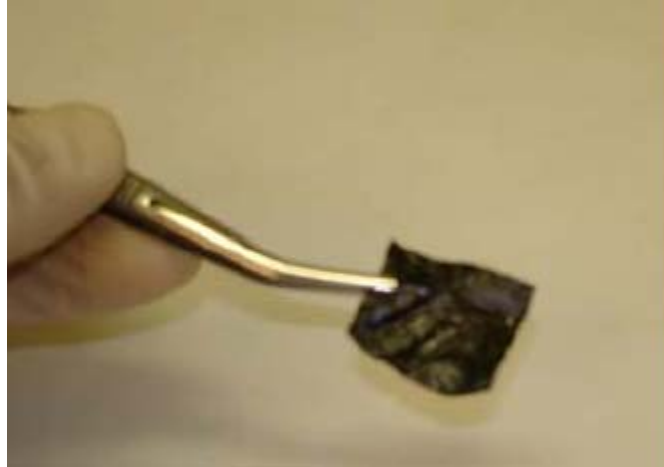
Figure 6-10: An example of a conformable free-standing LbL SWNT-PSS/PVA thin film after being etched from its glass substrate.
