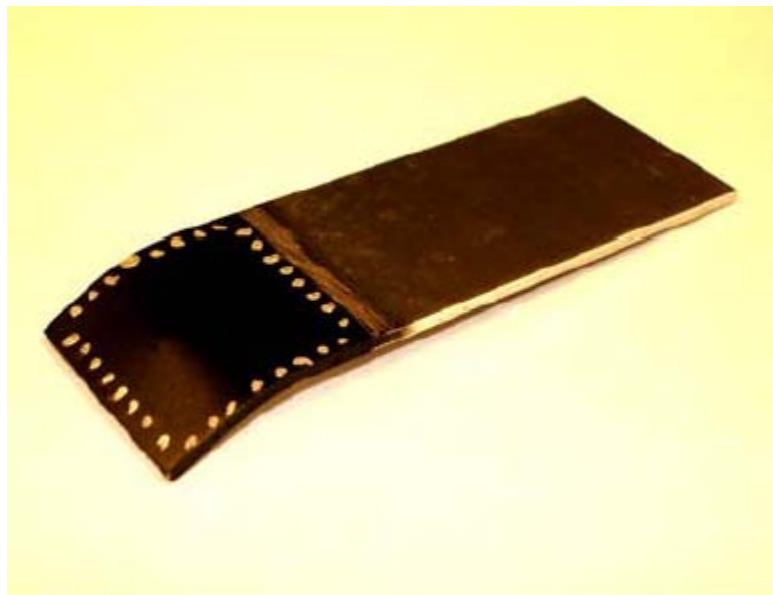
Figure 6-14: The specimen in Figure 6-13 is impacted with a tapered aluminum rod to cause bending and a bulge in the middle of the SWNT-PSS/PVA impact damage sensor.
