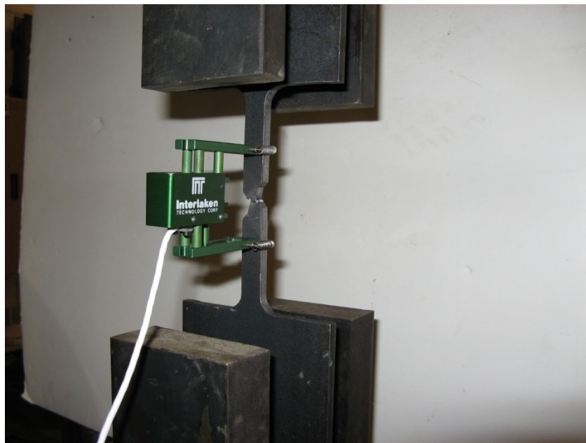
Figure 6.14 Specimen fractured after the test
