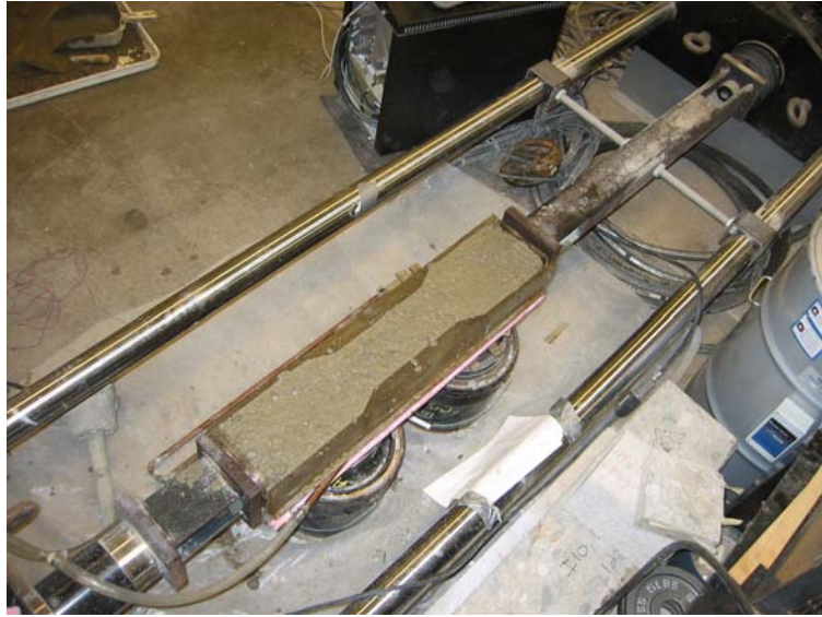
Figure 3.2 Top view of TSTM (a) schematic illustration of the apparatus; (b) specimens right after casting and prior to testing
