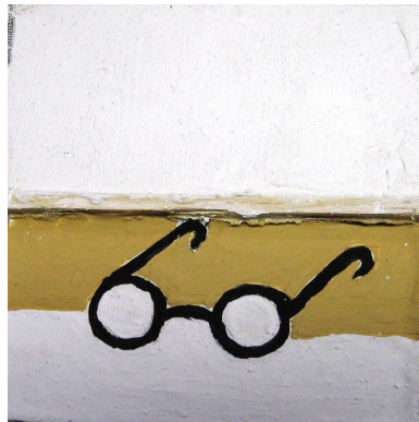
Figure V.16: Optical photograph of uncovered and covered sections of identical pairs of eyeglasses. Each section is 120 mm by 60 mm in dimension.
