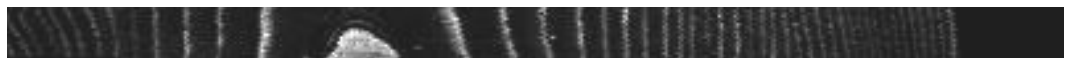
Figure IV.14: THz image of section of unvarnished pine 2 wood specimen (100 mm x 10 mm dimensions, 0.25 mm x 1 mm pixel size).
