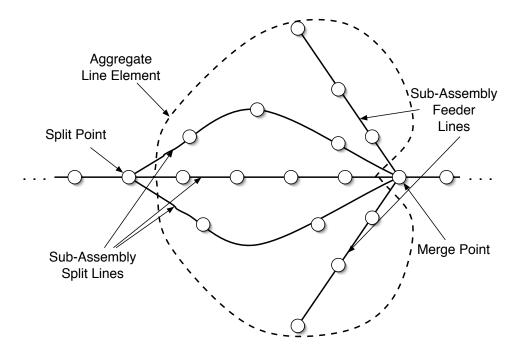
Figure 3.1: Partial Network Representation of a Production Line
