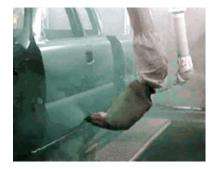
Figure 1.3: Primer coat application (Courtesy: General Motors Corporation, 2008c)
