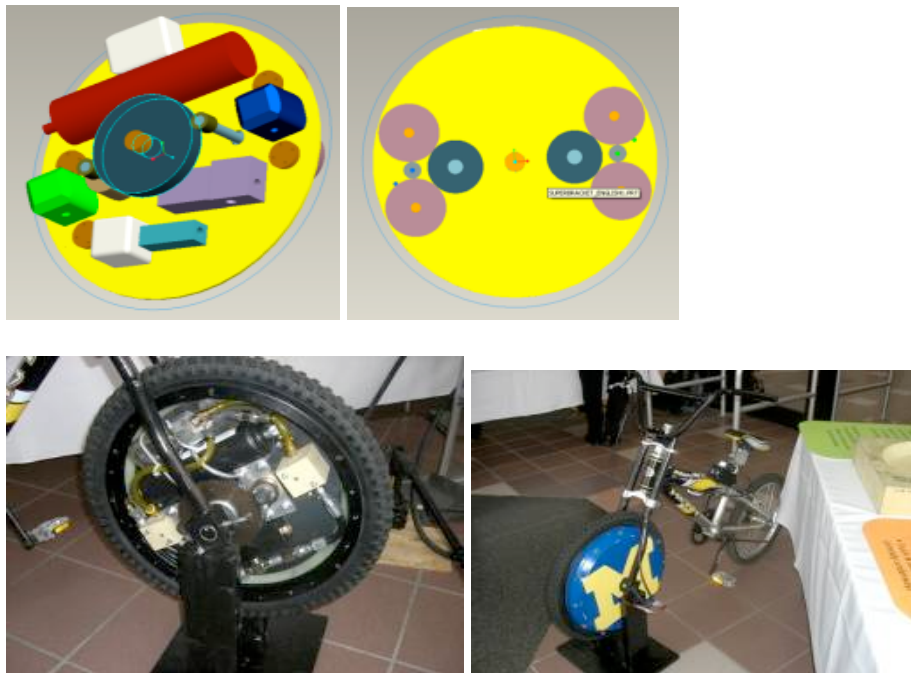
Figure 11: Final Concept – Engineering and Prototype Drawings for the Winter 202008 EPA bike hub
