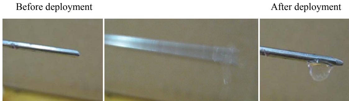
Figure 59: Test of fluid injection system on prototype device
