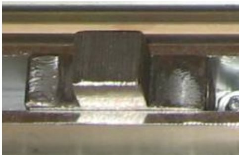
Figure 31: Completed square pin shown in its aluminum channel.
