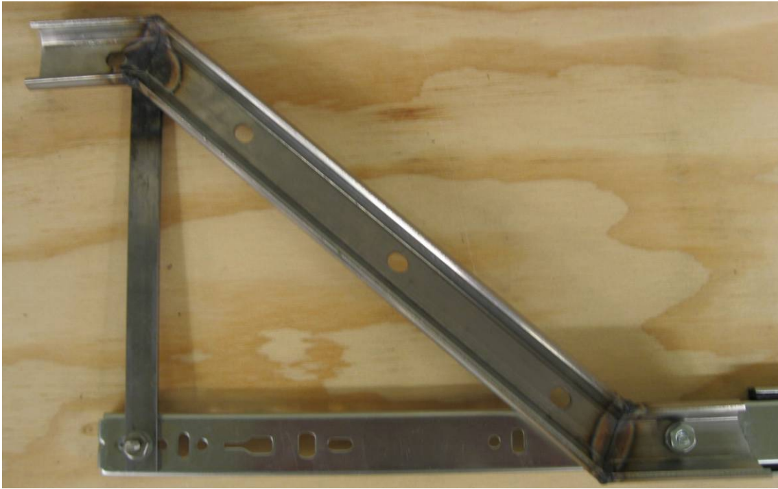
Figure 29: One completed track and connection bar shown attached to the slide.
