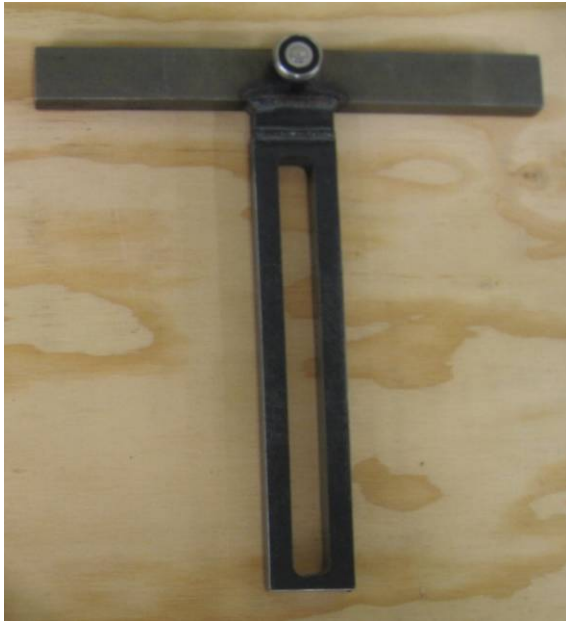
Figure 30: Completed T-bar. Note the added material as described above.
