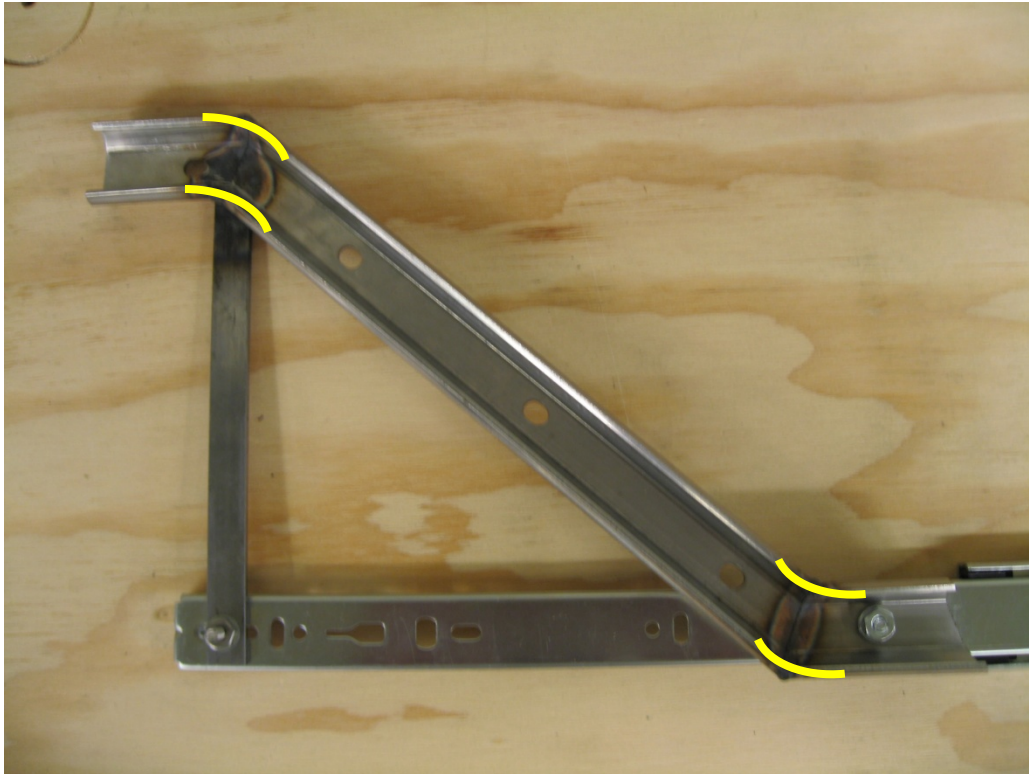
Figure 36: Corners to be rounded
