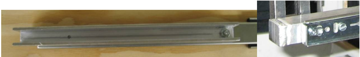
Figure 32: Completed aluminum channel shown mounted to the slide.
