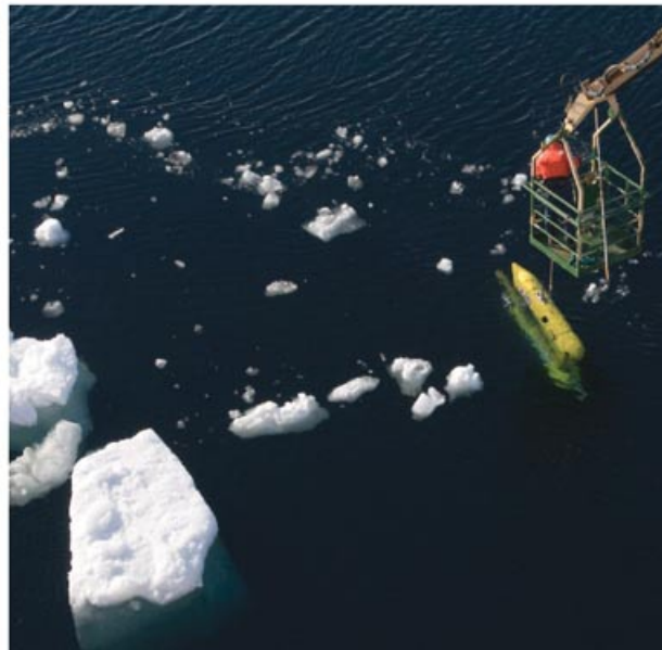
Figure 2. The size of open leads and density of the ice during AUV recovery varied greatly from dive to dive. Opening a pond sometimes also required moving the ship, temporarily precluding AUV communications. The AUV is barely visible in the left-hand image.
