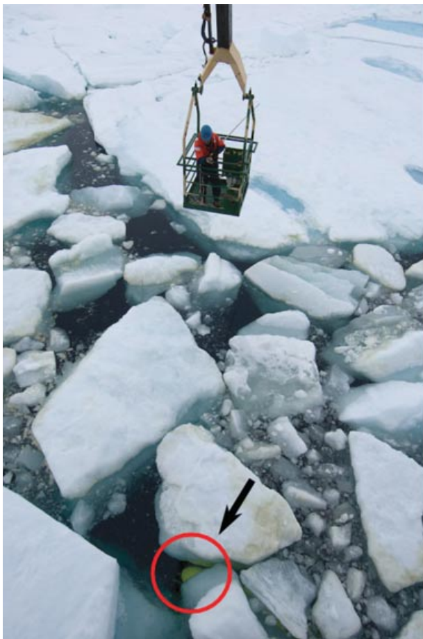
Figure 2. The size of open leads and density of the ice during AUV recovery varied greatly from dive to dive. Opening a pond sometimes also required moving the ship, temporarily precluding AUV communications. The AUV is barely visible in the left-hand image.
