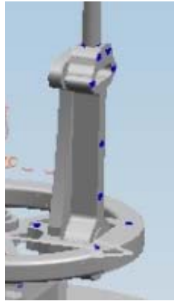
Figure 39: Pendulum and Stopper Plate on Large Device Eliminate Pinch Points and Limit Travel to 10° on Either Side of Vertical
