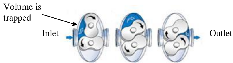
Figure 20: Air compression for a lobe compressor.
