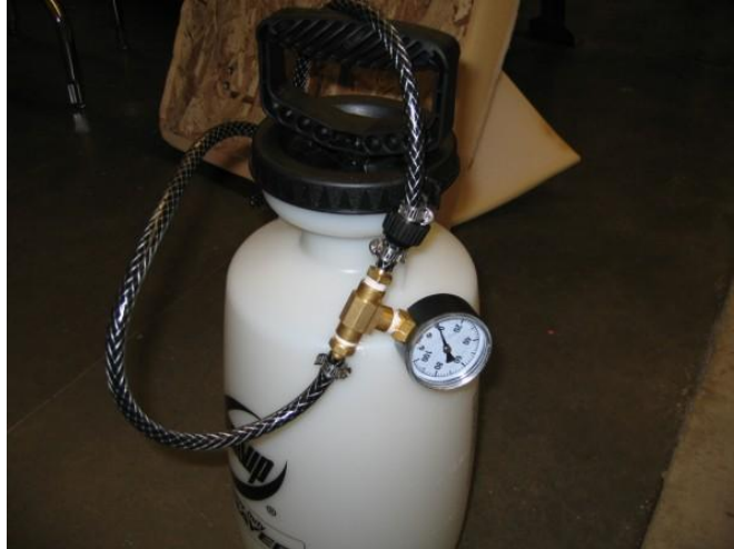
Figure 82: Water Tank Pressure Gauge Attached to Line
