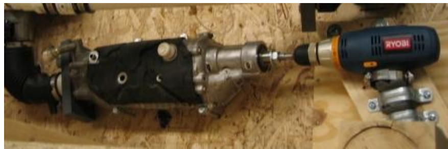
Figure 74: Compressor Shaft and Drill Chuck Must Align
