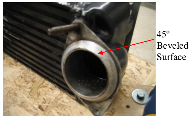
Figure 79: Intercooler Flange with Beveled Surface
