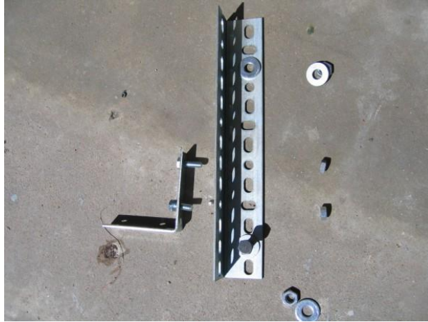
Figure 76: L-Bracket and Aluminum Rail for Intercooler Mounting
