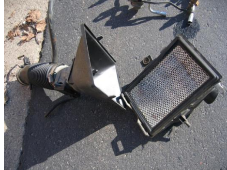
Figure 29: Air Box with Paper Filter
