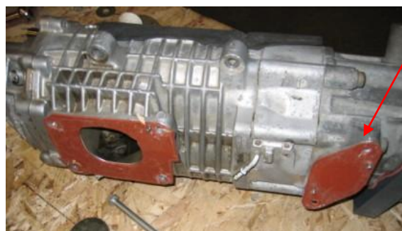
Figure 65: Bypass valve flange at inlet sealed
