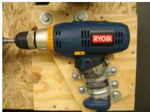
Figure 75: Support to Raise Drill to Proper Height
