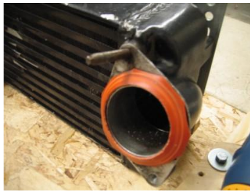
Figure 81: Rubber Gasket on Intercooler Flange for Adaptor
