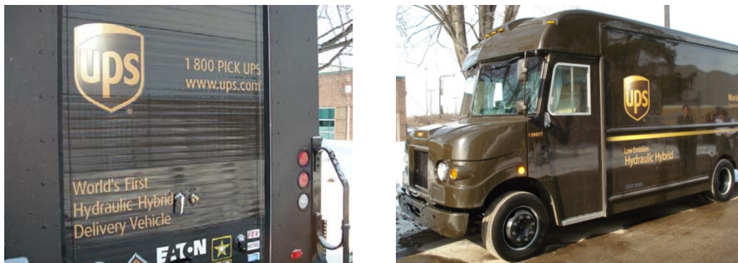
Figure 4.4: One of the first fully assembled hydraulic hybrid delivery vehicles.
