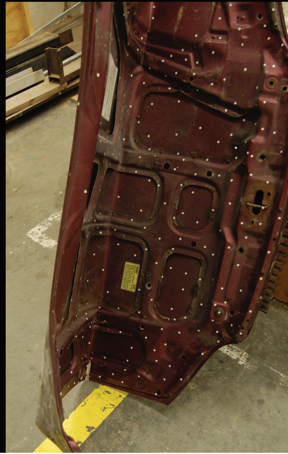
Dots were applied to surface of hood and scanned using a 3D digitizer. These points were then connected in a 3D modeling program to create a wireframe mesh. (shown to the left)
