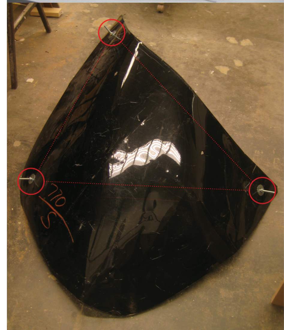
(Right) Location of bolts indicate points of triangle used to translate physical hood into digital modeling software.
