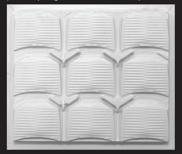
Once digitized, the hood was scaled down and a positive mold was made using MDF and a CNC router. The mold was translated to polystyrene using a vacuum former.
