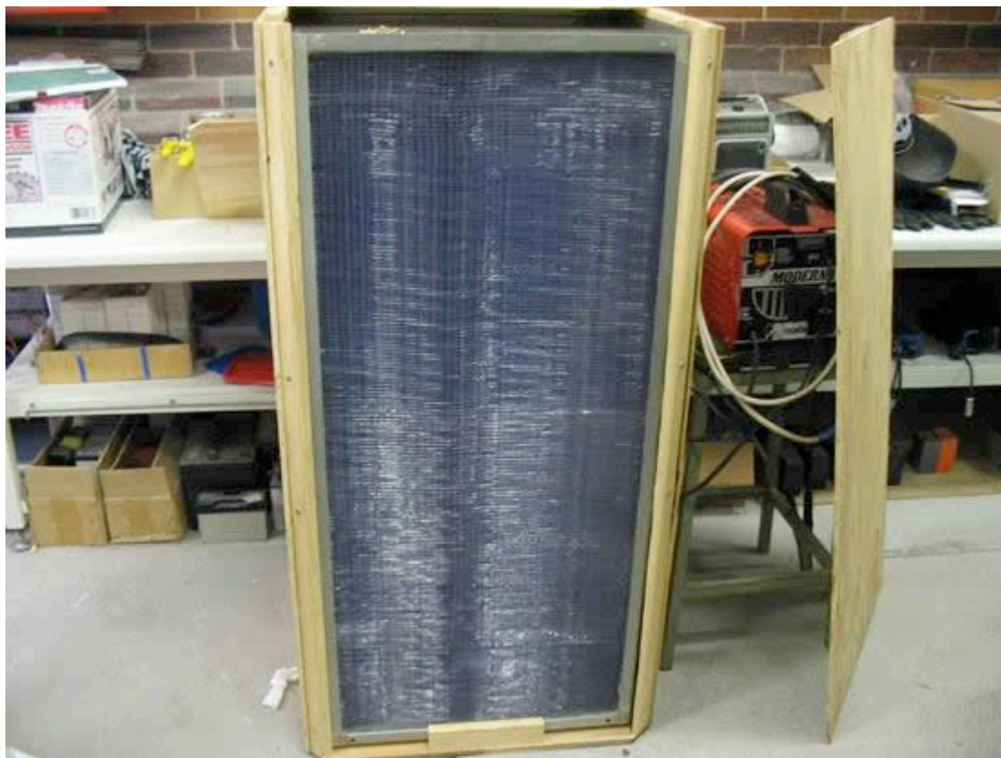
Photograph of 570 x 570 x 1175 mm cross-flow type PHE
