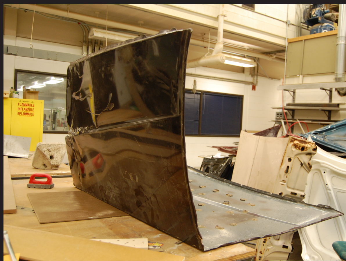
Hood is stripped of understructure and folded using a brake
