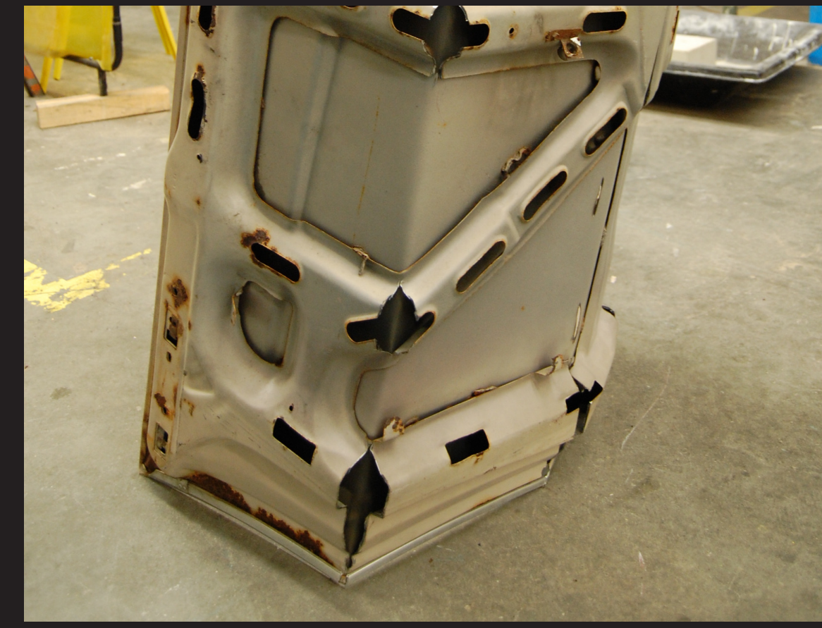
Perforation along hood rib structure allows for folding
