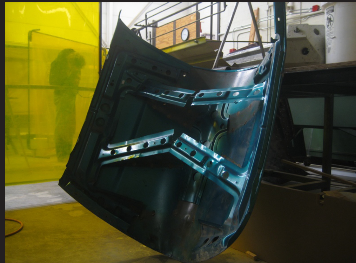
Hood understructure is cut and drawn together. Existing perforations, once translated within parametric software, can be considered increments for distance parameters. The effect of drawing the structural arms closer is bowing of the hood generating a larger section
