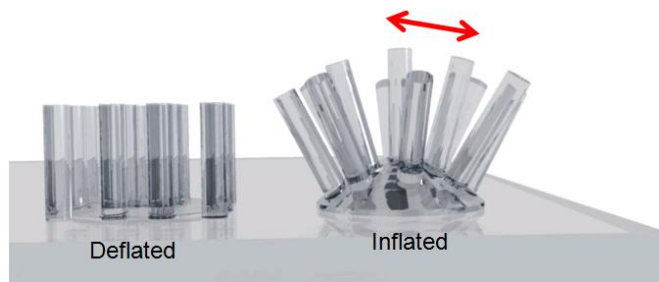
Figure 11: The inflated bubble spreads apart the protrusions that attached to it
