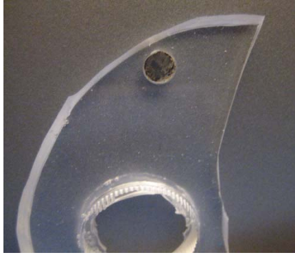
Figure 15: Test cut of the small upper hole using the laser cutter revealed its ability to successfully cut PDMS material
