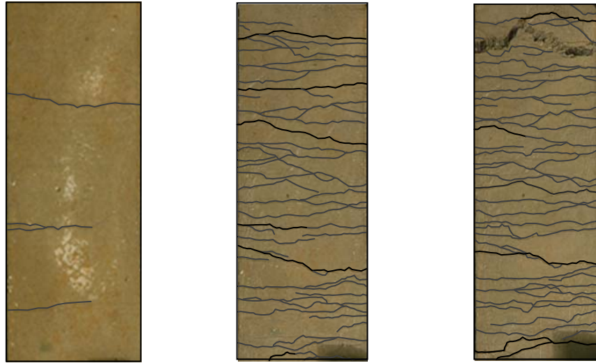
(a) First few cracks
