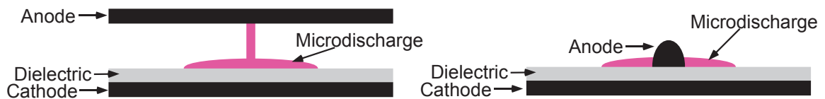
Figure 1.3: Schematic diagrams of the (a) volume discharge and (b) surface discharge DBD.
