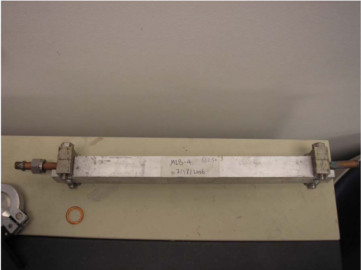
Fig. A-1: Noble gas sample tubes (standard refrigeration grade 3/8" Cu tubing) with stainless steel pinch-off clamps at either end.
