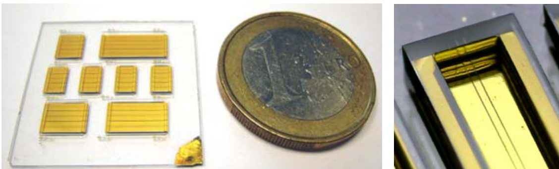
Figure 9-5: photograph and microscopic image of the fabricated CPW sensor chip
