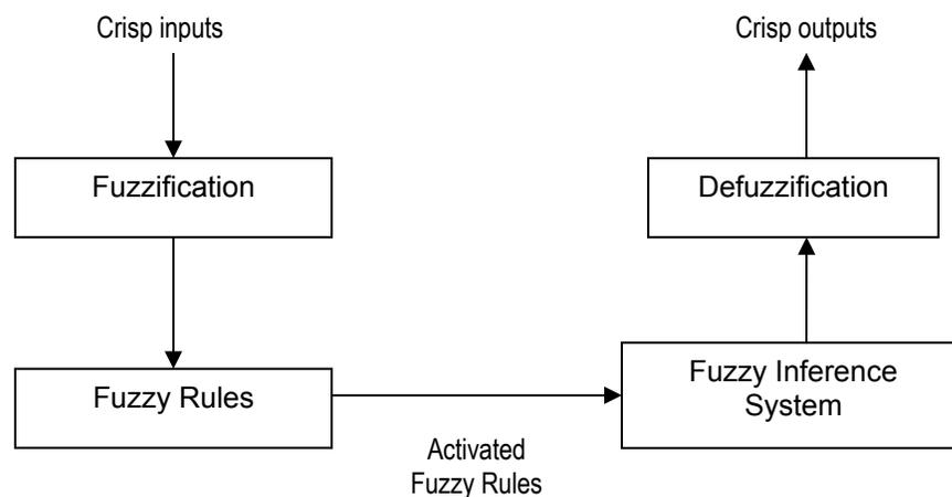
**Figure 6.1: Schematic of a Fuzzy System**
