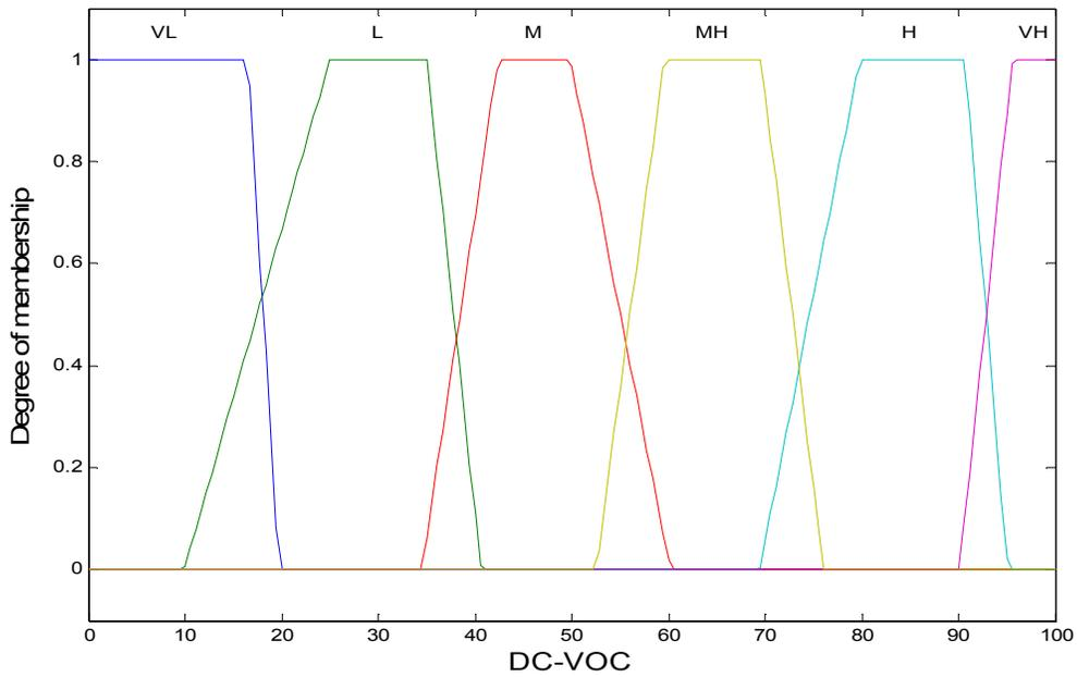
**Figure 6.13: Membership Functions for the Fuzzy Output Variable Damage Costs of VOC (DC-VOC)**
