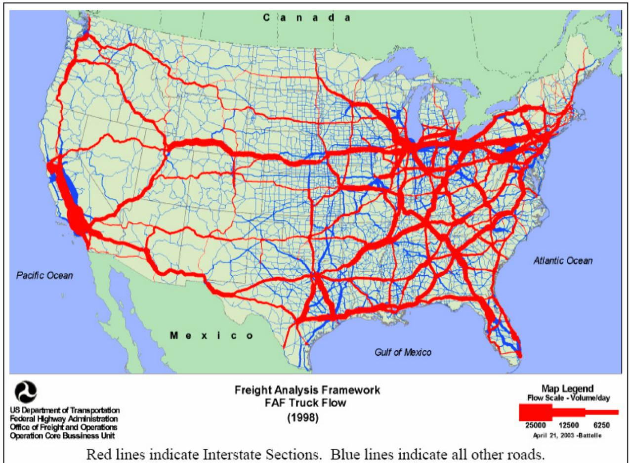
**Figure 4.2: Truck Flow and Highway Interstate Congestion**
