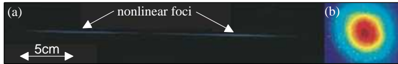
Figure 3.3: (a) Sequential filament structure in Ar at 870\text{mbar} as observed from plasma fluorescence. (b) Spatial mode after re-collimation.
