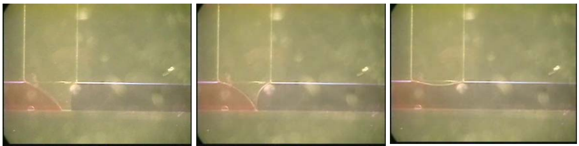
Figure 3-1. (a) A schematic of the use of 2D MBV to coalesce two drops. (b) The trapped air between two drops can be drawn off by a vacuum source connected to the MBV or by applying air pressure from the both ends to push two drops towards the center and the trapped air out to atmosphere via the MBV.
