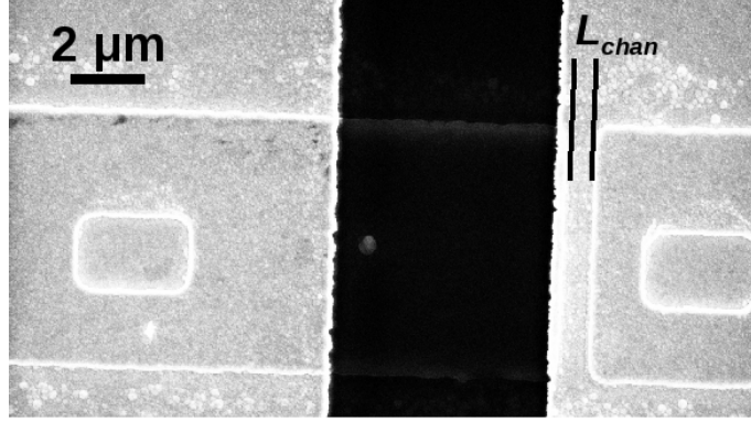
Figure 2.3: An SEM image of a 0.5 \mu\text{m} channel length lateral spin-valve.
