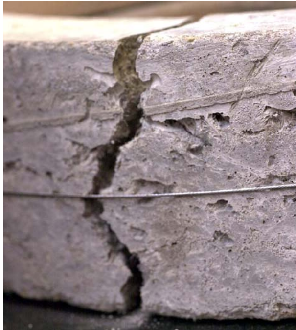
Figure 8.6: Localization crack of PVA specimen
