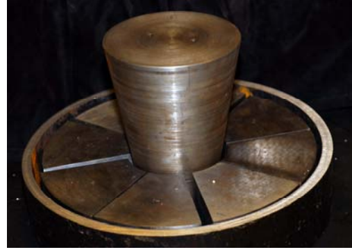
Figure 3.27: Ring HPFRCC setup
