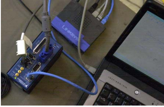
Figure 3.40: Image acquisition processing hardware (NI-CVS1453)
