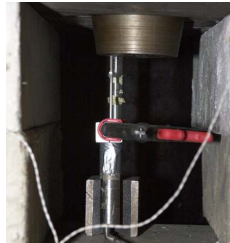
Figure 3.35: LVDT setup at cone wedge
