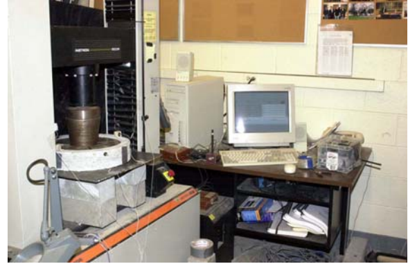
Figure 3.33: Testing machine and tensile ring setup
