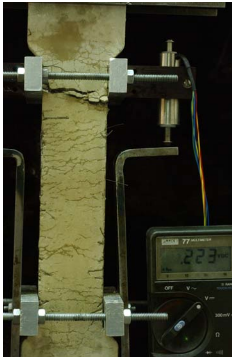
Figure 6.58: Typical failure crack in a tensile specimen reinforced with Torex fiber
