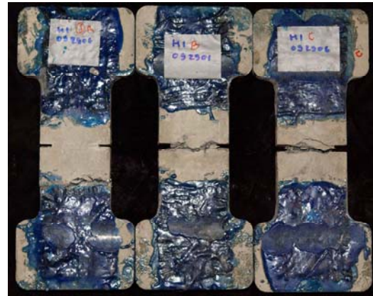
Figure 5.41 (b): Photo of tested specimens reinforced with 1.0% Hooked fiber
