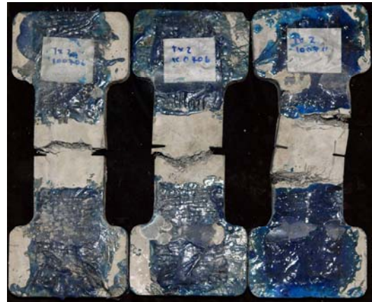
Figure 5.56 (b): Photo of tested specimens reinforced with 2.0% Torex fiber
