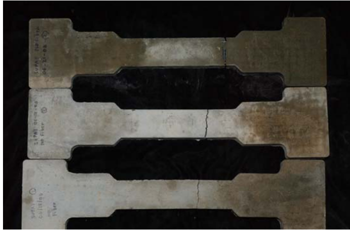
Figure 4.7: Dogbone specimen without fibers (specimen 4, 5, 6)
