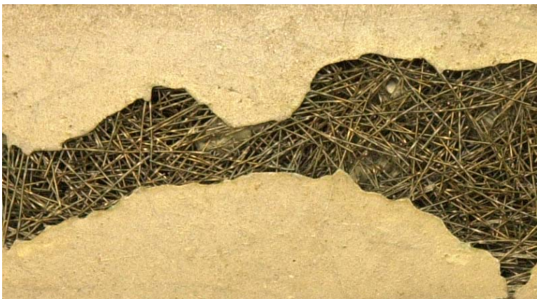
Figure A-5: SIFCON surface with large number of fiber in the specimens. (Torex)
