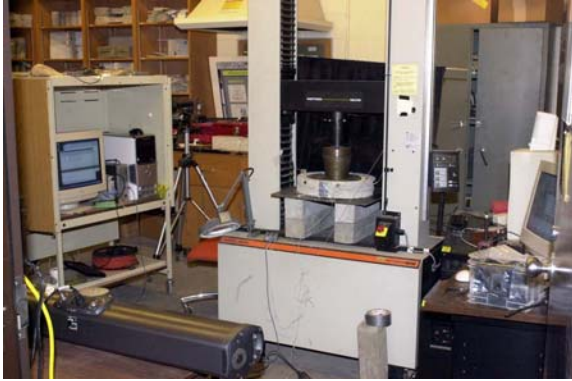
Figure 3.32: Testing machine and tensile ring setup
