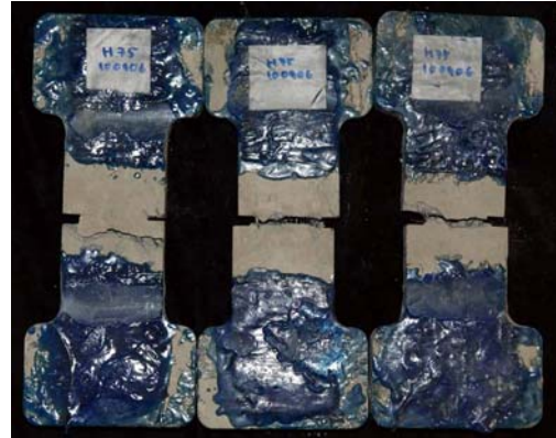
Figure 5.40 (b): Photo of tested specimens reinforced with 0.75% Hooked fiber
