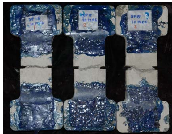
Figure 5.28 (b): Photo of tested specimens reinforced with 1.5% Spectra
