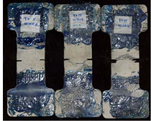
Figure 5.55(b): Photo of tested specimens reinforced with 1.5% Torex fiber
