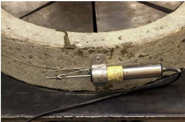
Figure 3.34: LVDT setup at specimen's surface
