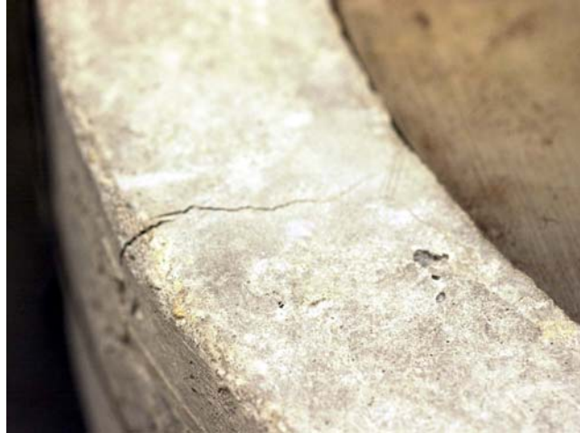
Figure 8.9- One of the four minor localization cracks
