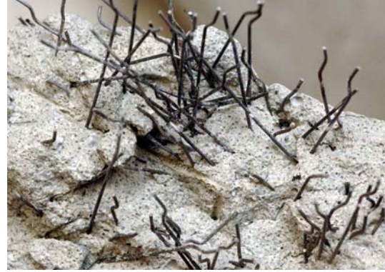
Figure 3.9: Hooked steel fiber in composites
