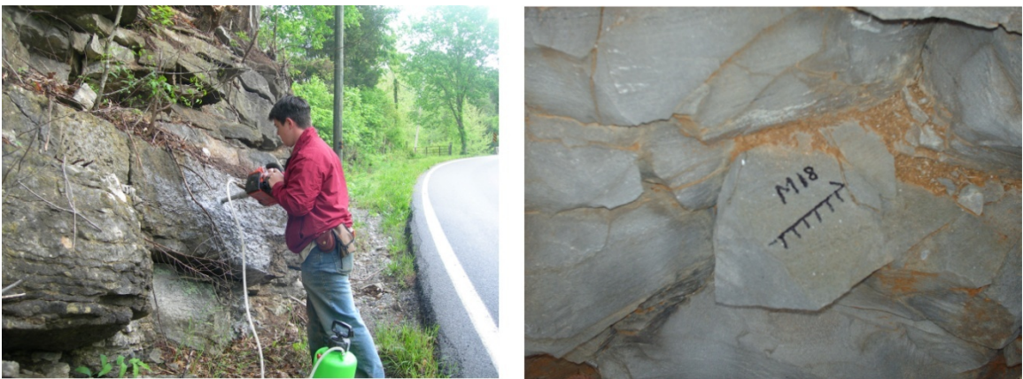
Figure B.1: Left: Drilling a sample for calcite twinning analysis. Right: Oriented hand sample.
