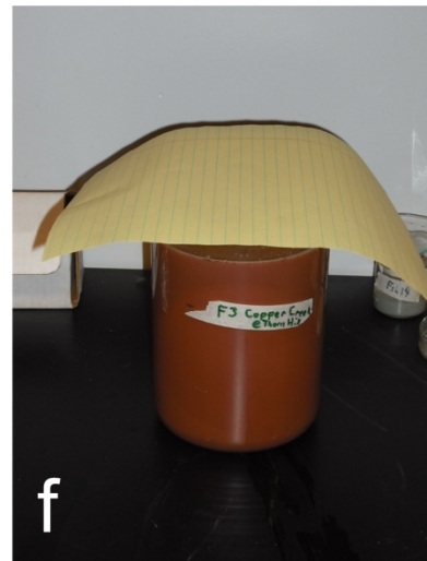
Figure C.2: Initial steps during sample preparation for IAA. (a) Gently crush the sample (b) pour into a beaker (c) fill with water (d) label the beaker (e) stir the sample (f) cover and allow to sit
