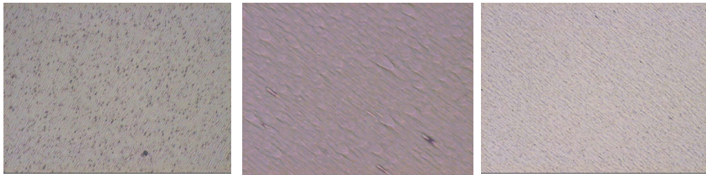
Figure 5.8: Optical microscope images of a a -plane GaN surface. (a) 1.2 \mu\text{m} , (b) 2.5 \mu\text{m} , (c) 2.5 \mu\text{m} thick a - GaN grown with high V/III ratio at the first growth step followed by a second step growth with low V/III ratio (from 2100 to 1070).
