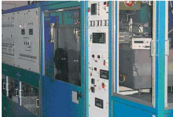
Figure 2.2: Image of the 3x2" Thomas Swan MOVPE system used in this work.
