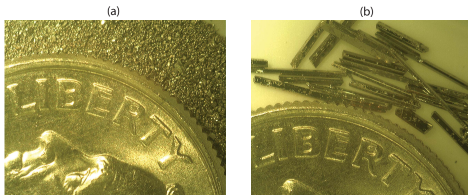
Figure 3.3: (a) A picture of single crystals of \text{Yb}_3\text{Pt}_4 grown using the temperature profile and element ratios in region 1 (blue, Fig. 3.2), next to a dime. (b) A picture of single crystals of \text{Yb}_3\text{Pt}_4 grown using the temperature profile and element ratios in region 2 (red, Fig. 3.2), next to a dime.
