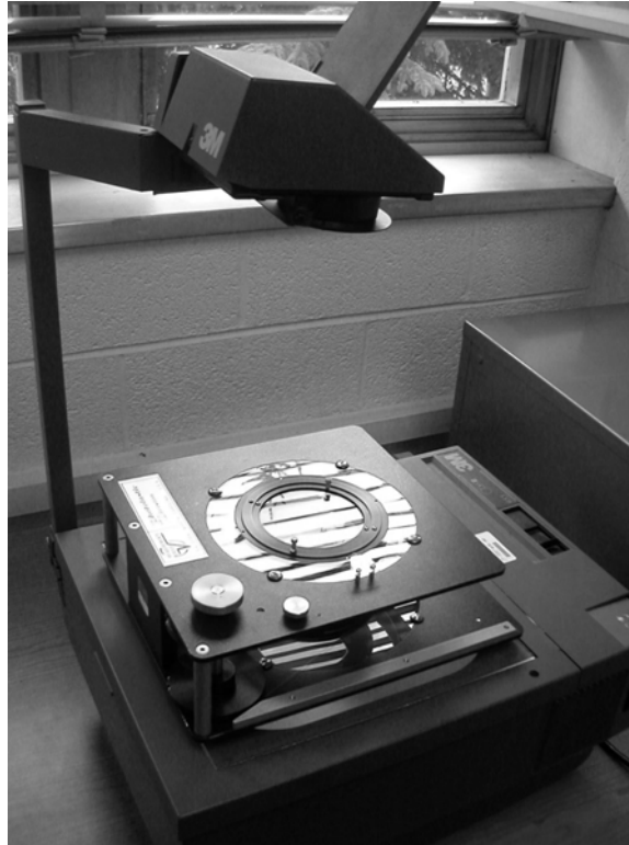
Figure 2.27: The Vishay Model 080 Teaching Polariscope. The polariscope uses an overhead projector as a white light source.
