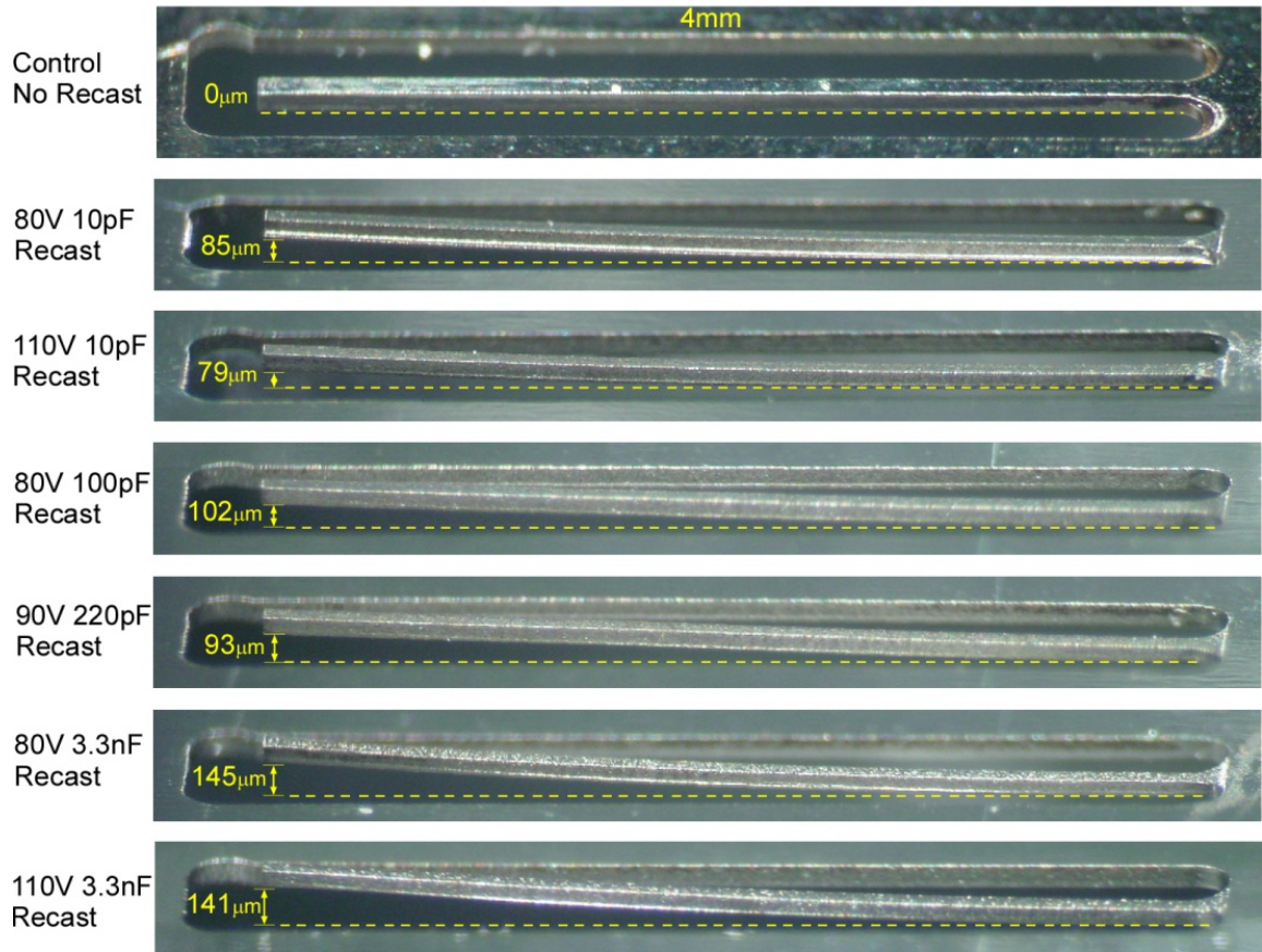
Fig. 5-4: Optical photos of 4mmX80 \mu mX75 \mu m cantilever beams under 7 different stress conditions.
