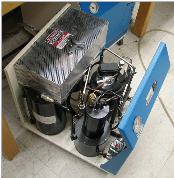
Figure 3.20: HC-2D compressor used in the cryogenic test facility (at UW-Madison).
