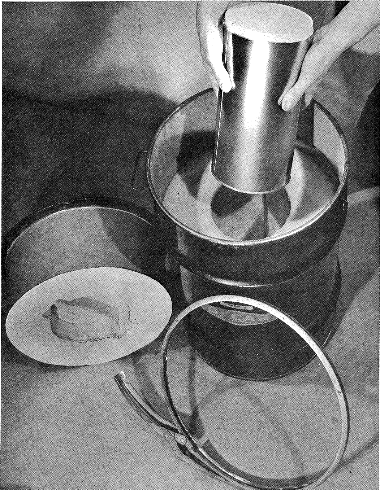
Figure 1. Specimen in disposable metal cylinder mold being placed in insulated autogenous curing chamber.
