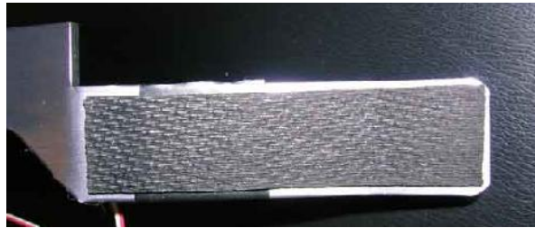
Figure 38: Padding Placed on Inside of Gripper
