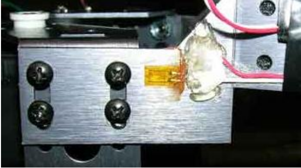
Figure 37: Strain Gauge on Outside of the Gripper
