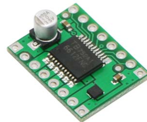
Figure 32. Motor driver used to control the DC motor.
