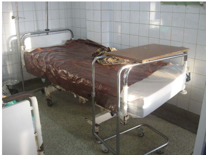
Figure 15: Corrosion and rusted frames of current beds in Ghana.
