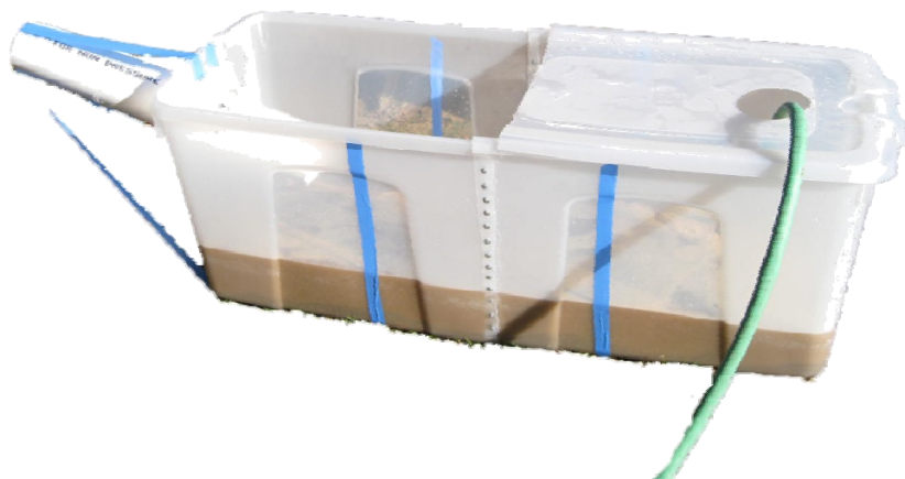
Figure 34: Schematic of testing rig sectioned off into 3 sections for analyzing local mixing
