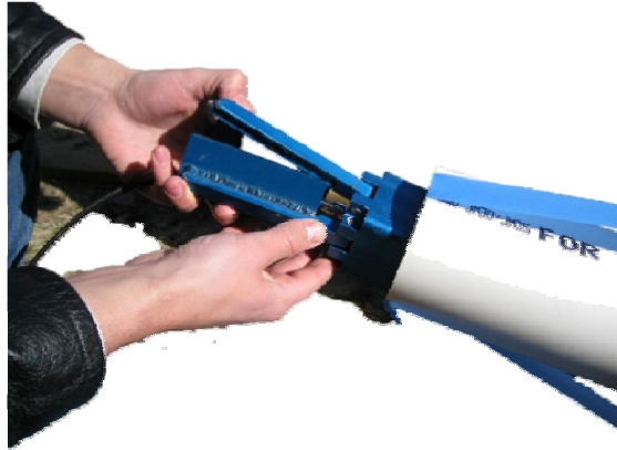
Figure 35: Insert the collapsed mixer into 4" diameter pipe
