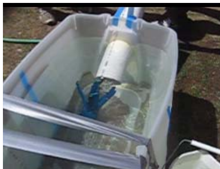
As mixer rotated clockwise, fins opened up easily
