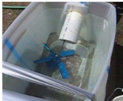
As mixer rotated clockwise, fins opened up easily
