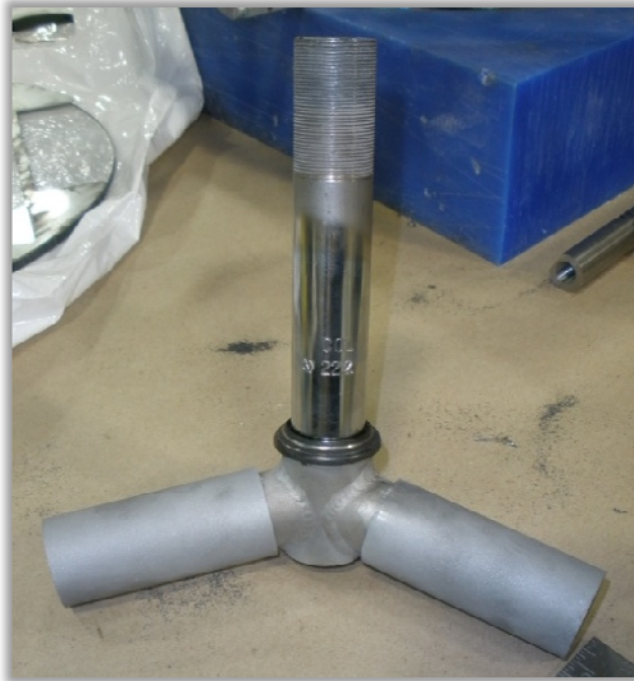
Figure 27: Horizontal fork members prior to welding
