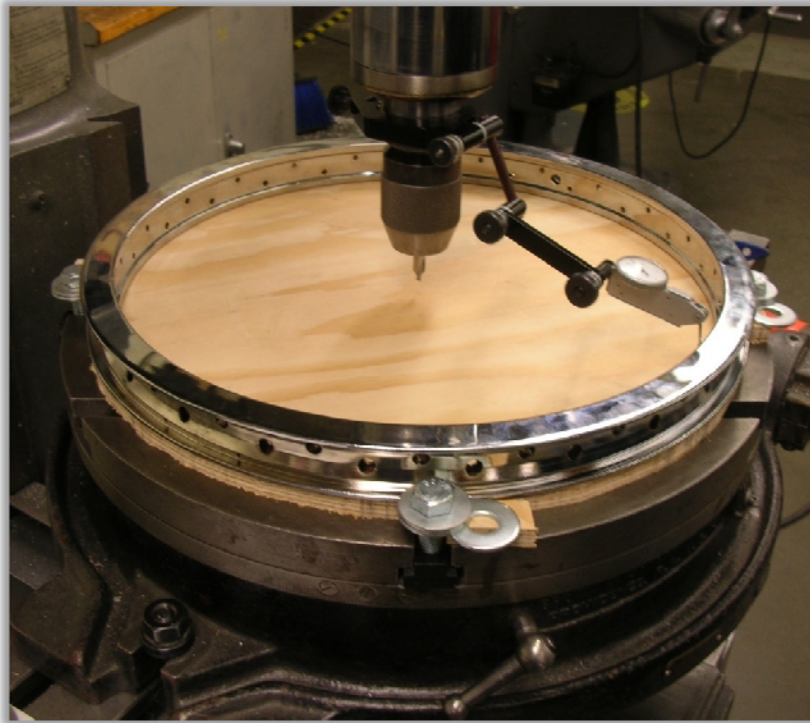
Figure 26: Aligning the rim on the mill in the ME Shop using a dial indicator
