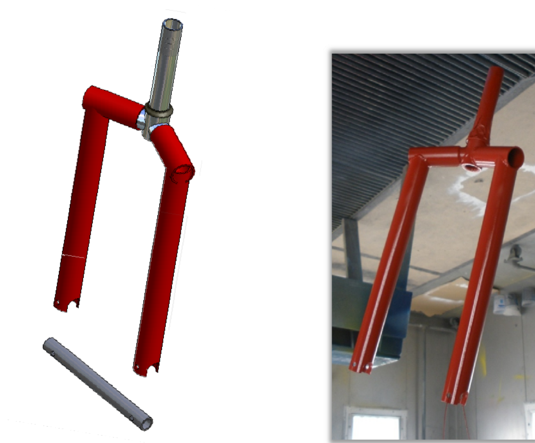
Figure 29: Front fork – From CAD model to reality
