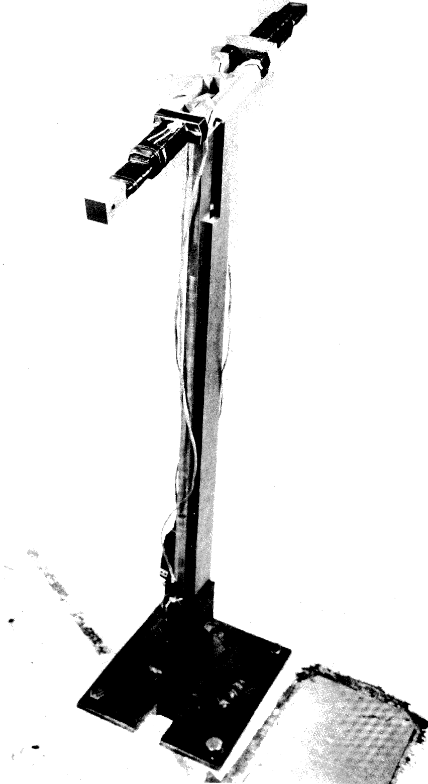
Figure 12. Fixed Mount Installed in Wind Tunnel.
