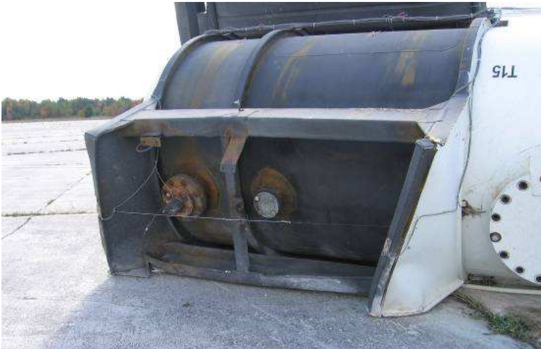
Figure B-22. Rollover protection devices after the crash
