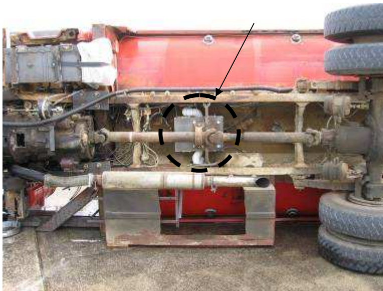
Figure 7. Inertial guidance unit on the single-unit truck It was mounted between the frame rails for protection.
