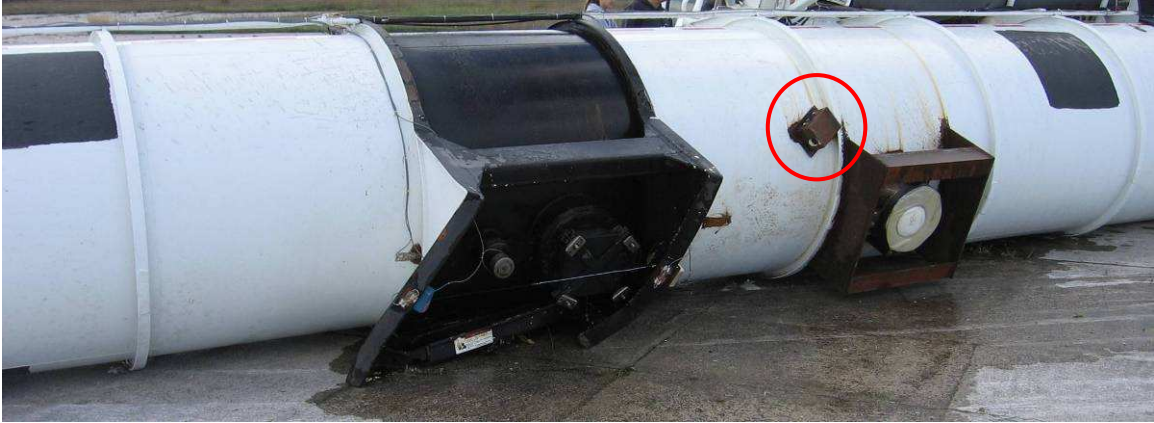
Figure C-6. The housing for the camera looking at the rollover protection device is in the circle. The GPS antenna is visible below and to the right of the camera.
