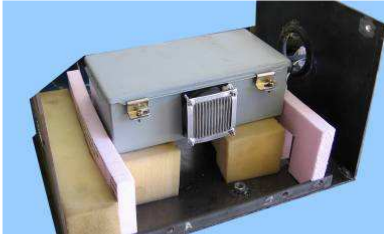
Figure 8. Support for the inertial navigation system
