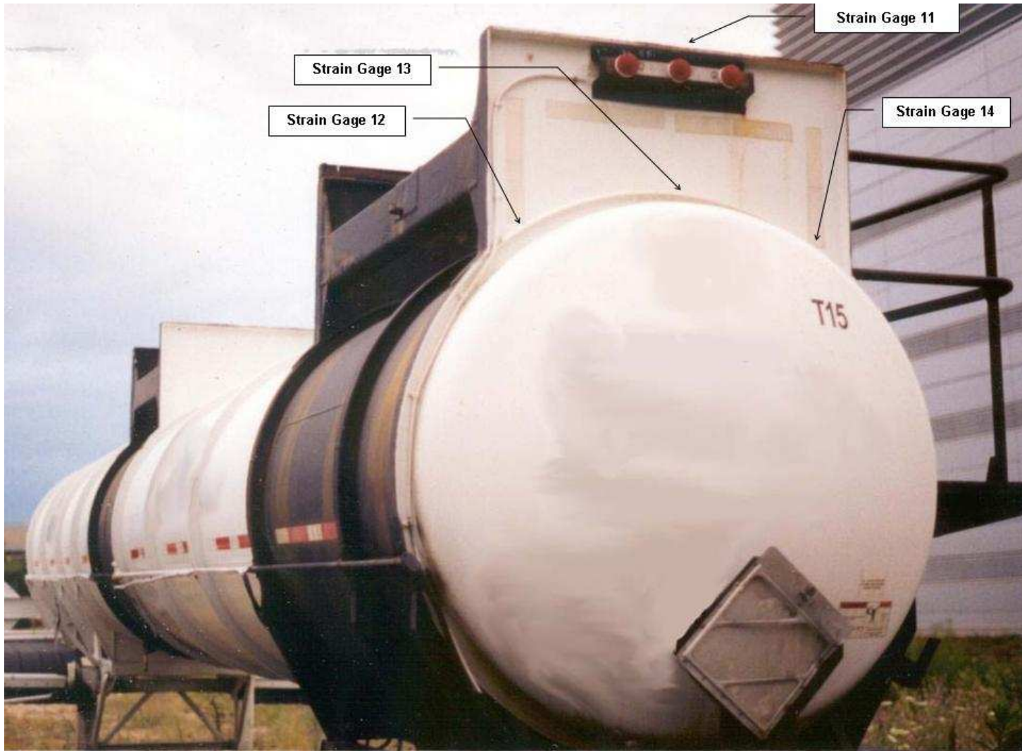
Figure B-1. Strain gage locations on the rear of the semitrailer
