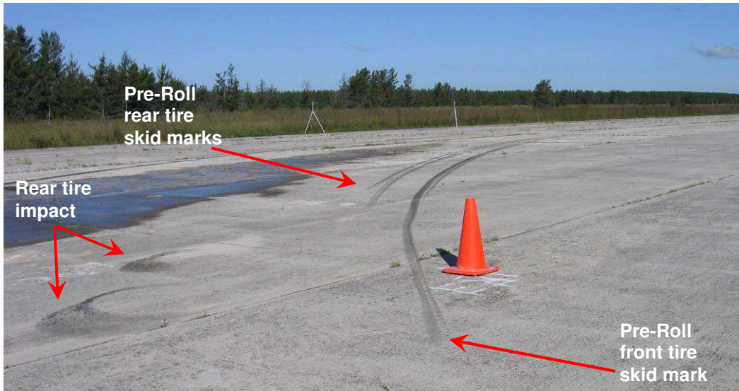
Figure 15. Skid marks from the third rollover
