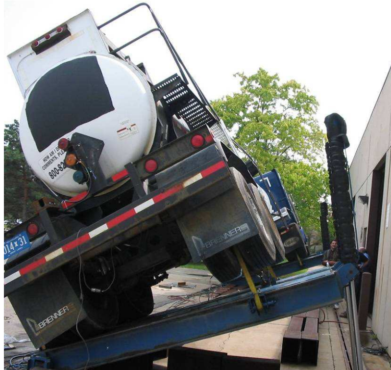
Figure 5. Tractor semitrailer on the tilt table
