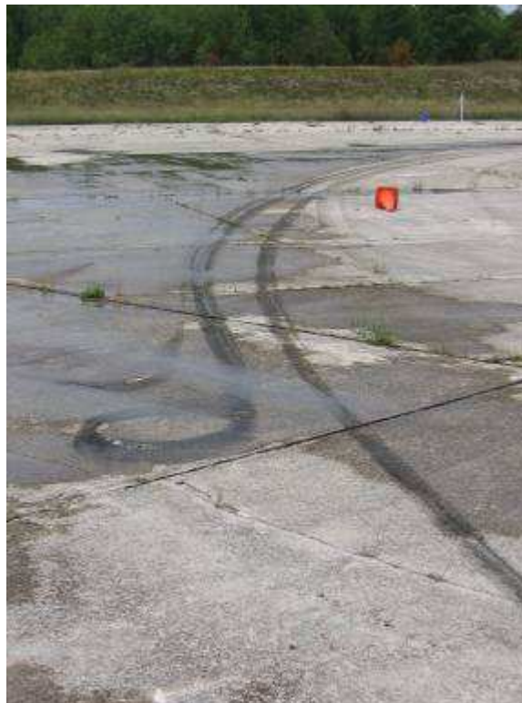
Figure 14. Skid marks from the first rollover
