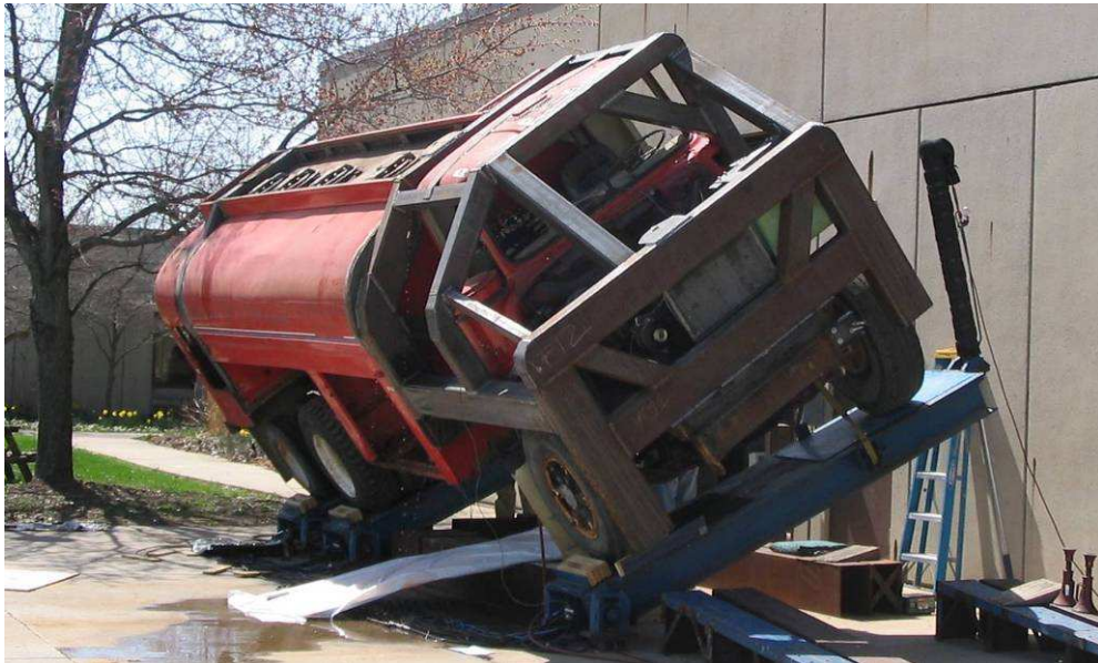
Figure 2. Single-unit truck on the tilt table
