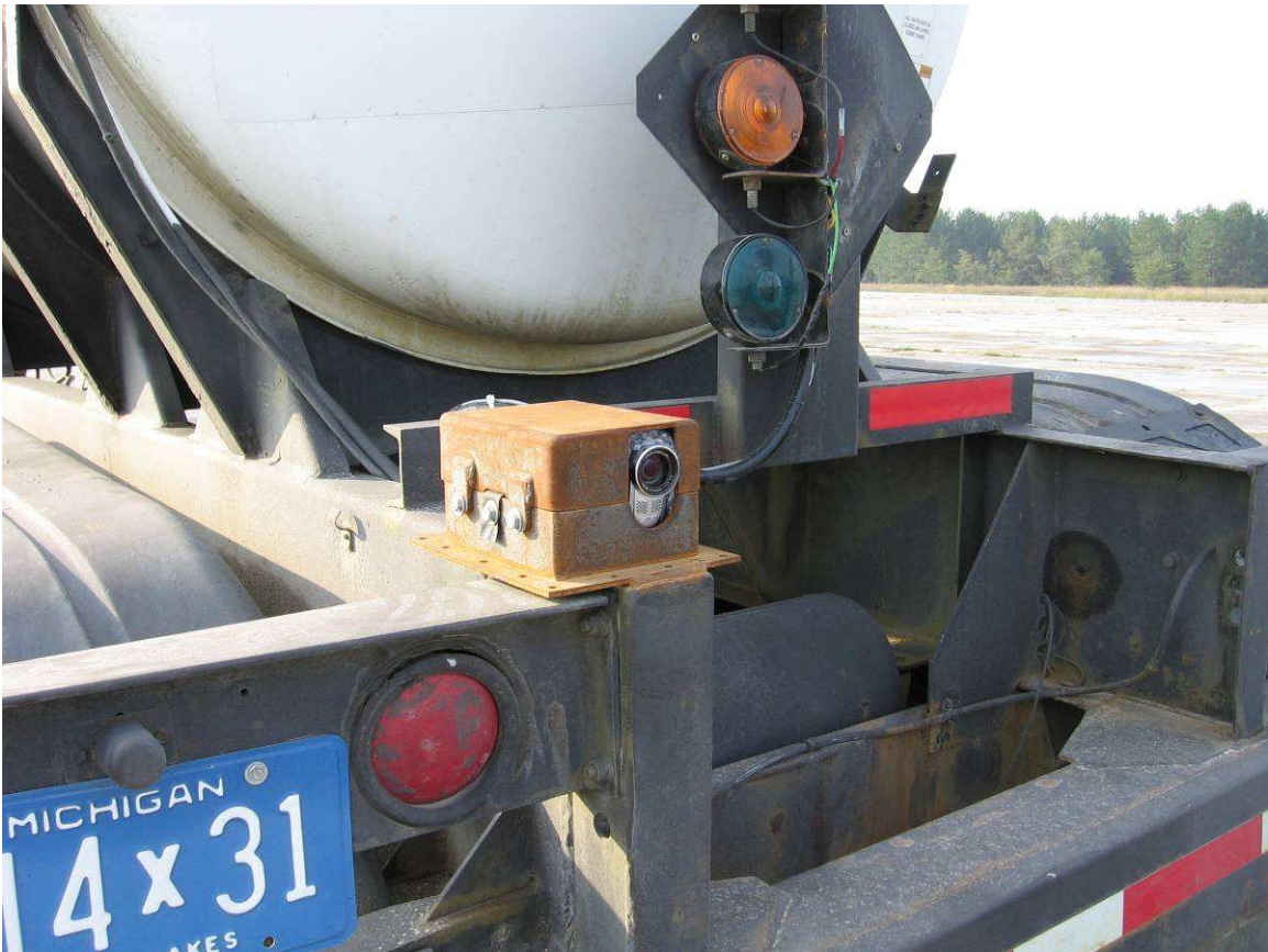
Figure C-7. The rearward-looking camera on the trailer.
