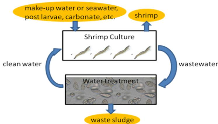
Figure 1 Schematic of a recirculating aquaculture system consisting of shrimp culture system and water treatment system.
