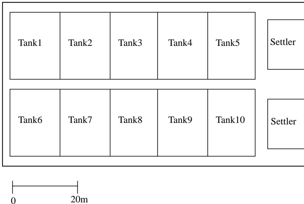
Figure 5 Layout of Oceanic Institute Farm Building, including 10 tanks for shrimp culture and 2 settlers for water treatment.
