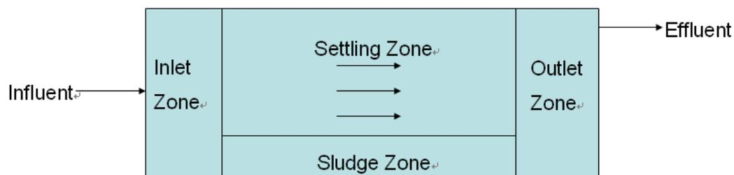
Figure 6 A schematic of four principal zones of a rectangular continuous flow sedimentation basin
