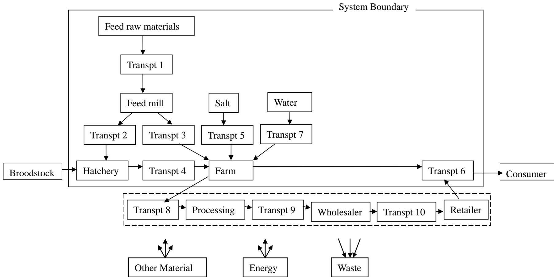
Figure 4 Detailed life cycle of recirculating shrimp aquaculture system, which highlights the scope of this thesis (excludes brood stock production and consumer stages).
