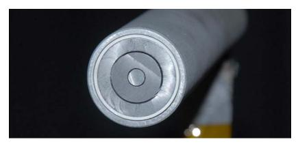
Figure 3-25 Photograph of the AFRL nested Faraday probe shown in the 0.5 mm gap width configuration.
