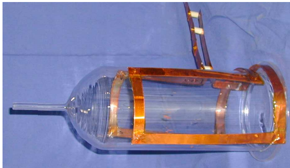
Figure 3.3: Photograph of the Boswell-type antenna. The antenna is wrapped around the quartz tube used in the helicon source.
