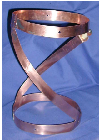
Figure 3.5: Photograph of the double-helix, half-wavelength antenna.
