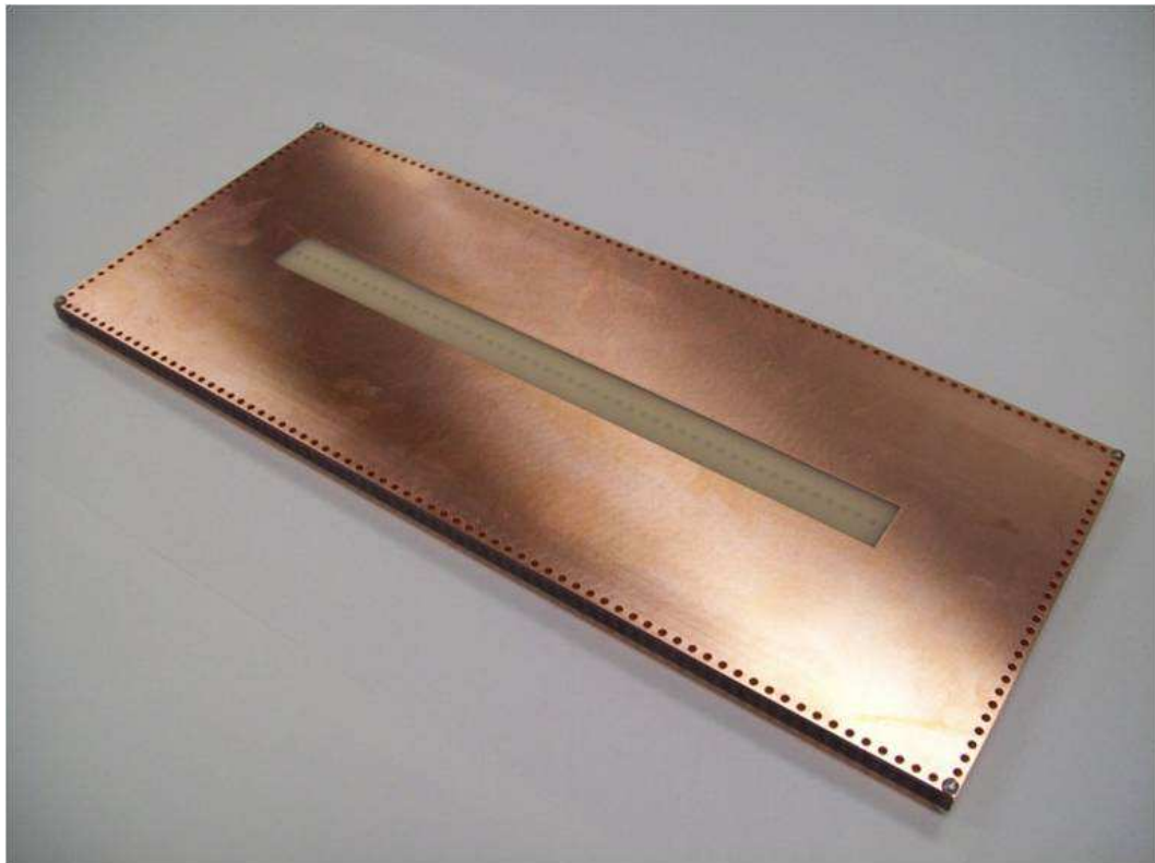
Figure 3.15: The fabricated Shielded parallel plate resonator-backed slot antenna using PCB technology.
