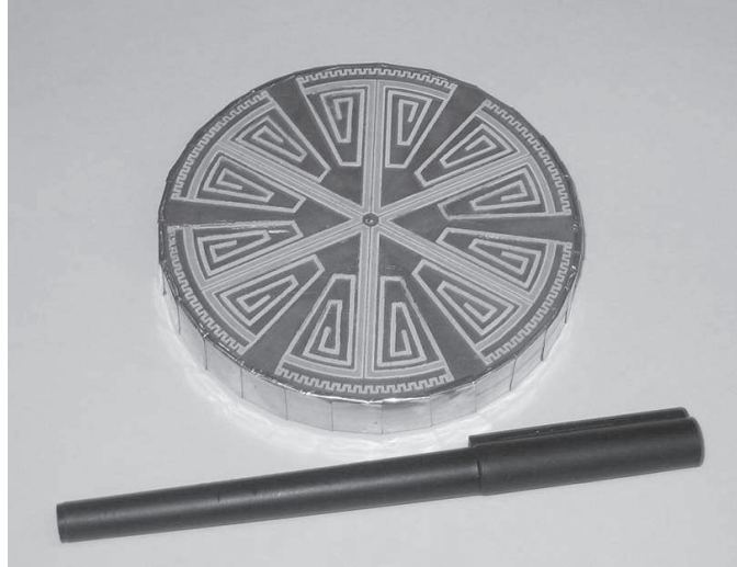
Figure 4.6: Photograph of the fabricated of the reduced-size-cavity-backed composite slot loop antenna. The coaxial feed is not shown.
